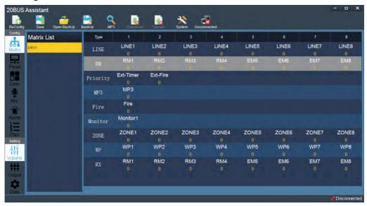
Volume setting includes matrix list and signal & port information. Double click the port which you want to adjust volume and will appear the new volume control windows as below. Then volume gain is from 0-20dB, the treble and bass EQ is from -5dB+5dB.
