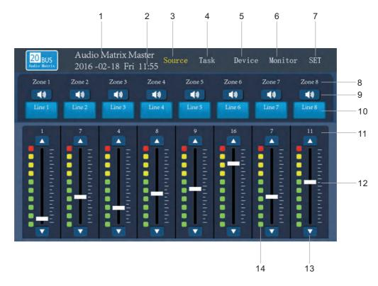
The main touchscreen on the matrix display the matrix name, date & time, zone name, audio source and volume information. On this screen, you can control the select the audio source, set the volume and mute for each zone.
