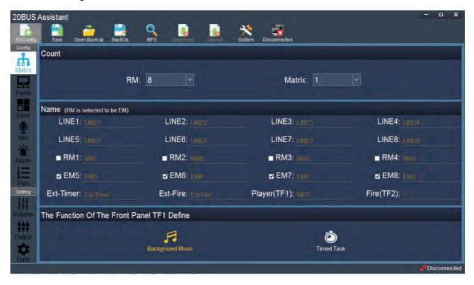
The matrix config menu screen use to set the general configuration of the PA system. It includes the matrix quantity, remote microphone station name and quantity, matrix input name, priority of remote microphone station, EXT-Timer name, EXT-Fire name, Micro SD1(TF1) name and its function define.
