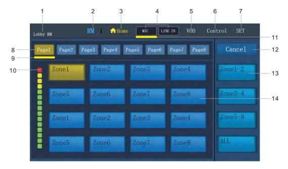
The main touchscreen of remote microphone station display the name, EM/RM priority, audio source, control, set up and paging zone selector etc. When a paging is needed, select your audio source first and then select the zone which you want, press talk button to start a paging (Push on, push off mode or Push to talk mode can be preset).
