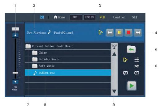
The VOD screen on the microphone station use to play the audio files in the micro SD card. Select the zone first, press talk button to page status, select and play the audio file to related zone.
